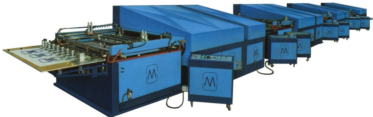
example of 4 colours line equipped with hot air dryers and final cooling modules
